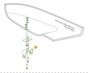
Feed the wires through the cable grommet and assemble the Bracket • with Bracket •.
