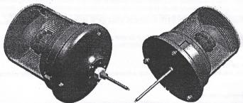
The 3 bolt and 1 bolt beacon have 13 flash patterns. To change the flash pattern, momentarily touch the blue cable to the negative.
